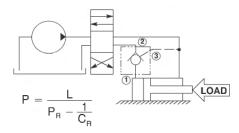
2) Pilot check on the rod end of the cylinder with a load extending the cylinder rod.
