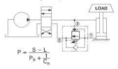
2) Counterbalance valve on the rod end of the cylinder with a load extending the cylinder rod.
